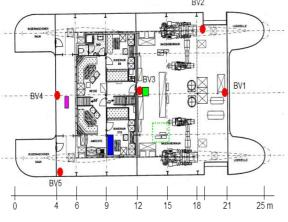
Accelerometers position on the main deck of the *Duhnen*.
