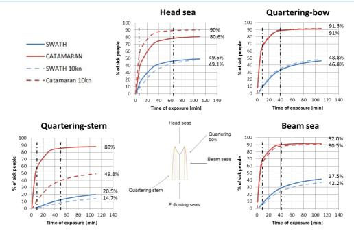
Comparison of motion sickness incidence of three crew transfer vessels with different hull forms
