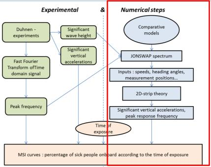
Comparison of motion sickness incidence of three crew transfer vessels with different hull forms
